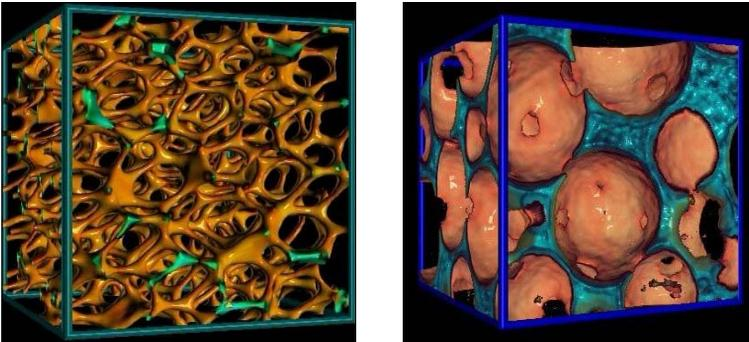
Fig. 19. Images of open-cell aluminium foam (left) and close-cell polyurethane foam (right) obtained by tomography.<sup>78</sup>
