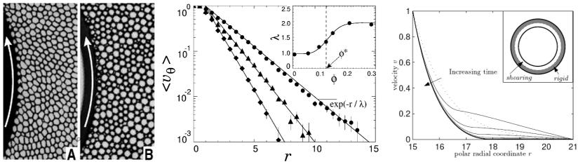
Fig. 14. *From left to right:* Experimental Couette setup for dry and wet foams; Exponential decrease of the tangential velocity across the gap (reprinted figures with permission from<sup>27</sup> Copyright (2001) by the American Physical Society); Prediction of the velocity profile by a continuum model.<sup>23</sup>
